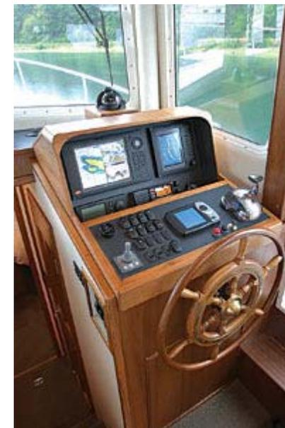
*The teak dash (above) at the lower helm station is recessed to cut down on the glare on the chartplotter screens. (below) The saloon is bright and airy, and features a reconfigured galley.*
